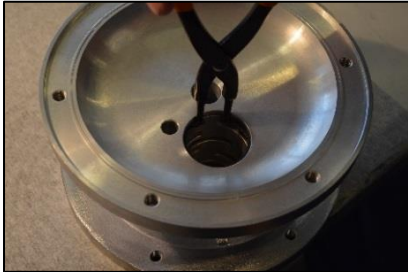
Fig. 3.6.1 Before inserting the air valve [61], insert the circlip [27] on one side of the centre block [12].
