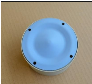
Fig. 3.6.3 When screwing in the diaphragms [15] on the shaft [16], the holes in the diaphragms must align with the holes in the centre block [12]. Sometimes it is necessary to turn the diaphragm back a little bit in order to align the holes.
