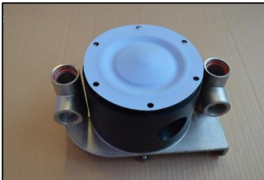
Fig. 3.7.3 Lift the loose manifolds [13] and centre block [12] from the second housing [11].
